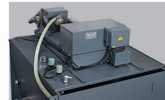
1. Magnetic separator 磁鐵過濾機 (0.02mm) 2. Paper filter 紙帶過濾機 (0.02~0.005mm)
