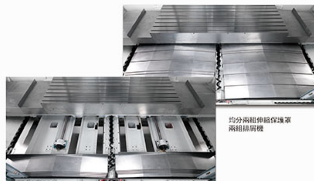
Y軸前後兩支鋼珠螺桿 Y軸三組捲屑機以利排屑
