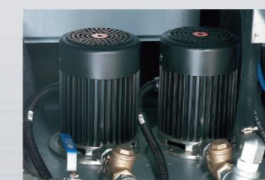
Dual vertical coolant pumps are concealed inside the machine to provide for a compact design.
