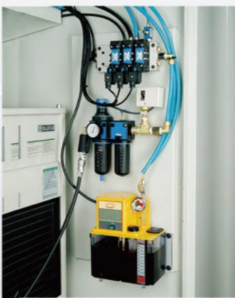
Equipped with high reliability lubrication pump and solenoid valves.
