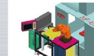
It unloads them inside the processing machine and grips the completed workpieces back to tray.
