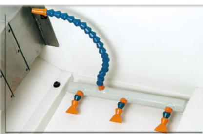
Rear wash-down nozzles makes chip clean up easily.
