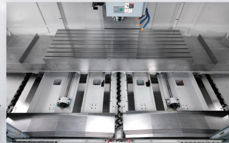
Two separated telescopic covers stand side by side and enable to clean up chips
