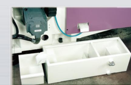
Oil collector: Separating for oil and water
