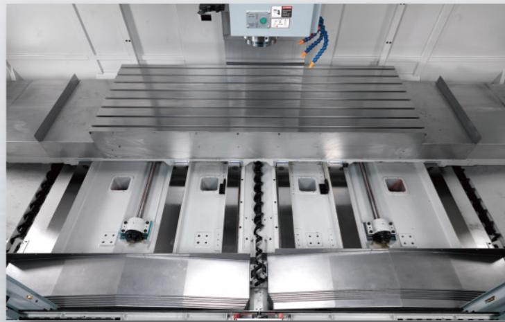
MCV-2510/3010 Y axis front/rear has two ball screws and three chip augers.
