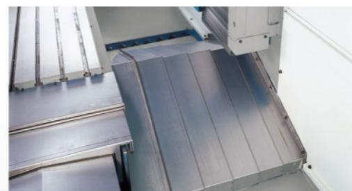
Slope telescopic cover to protect the guide ways
